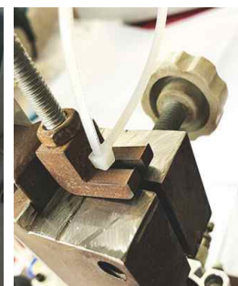
▶ 插入力測試、拉伸強度試驗 Insertion force testing and Tensile strength testing
