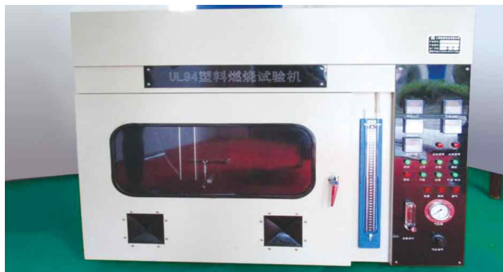
▶ UL-94 塑料燃烧试验机 UL-94 plastic combustion tester-flame resistance
